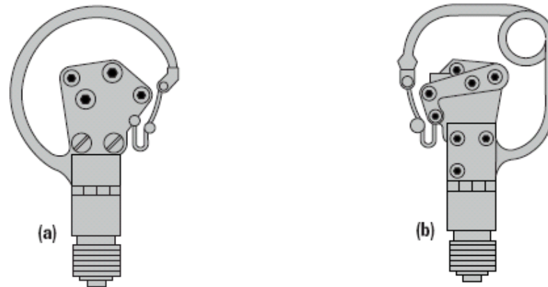
Fig. 12.6.1 'C'-shaped (a) and coiled (b) Bourdon tubes
