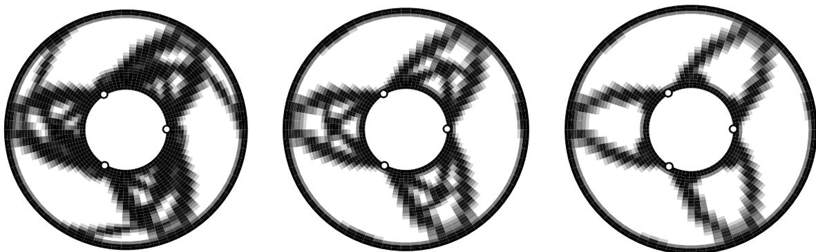
Fig. 8. Possible optimum topology for disk structures under mixed load.
