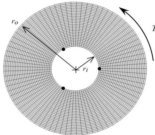
Fig. 1. A finite element model of a hollow disk under torsion.
