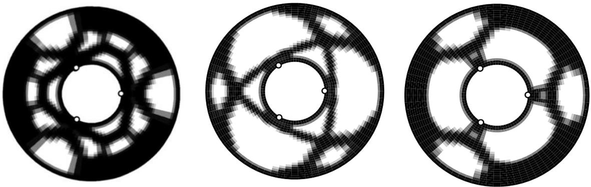
Fig. 7. Possible optimum topology for disk structures under radial load.
