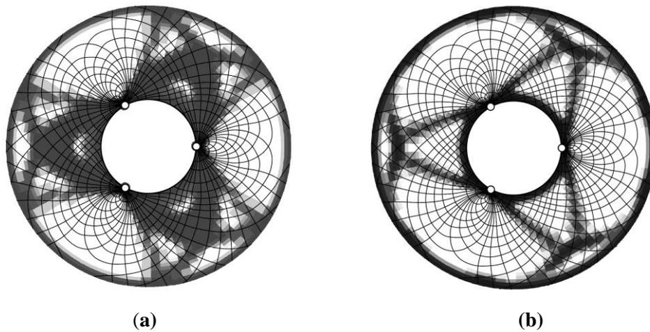
**Fig. 5.** Comparison of principle stress trajectories of the initial disk to (a) topology from iteration 20 and (b) final topology from iteration 35.
