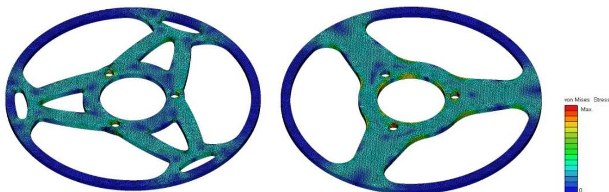
Fig. 4. Stress simulation of disk structures with optimum topology under torsion. (a) Optimum disk. (b) Arbitrary designed disk.
