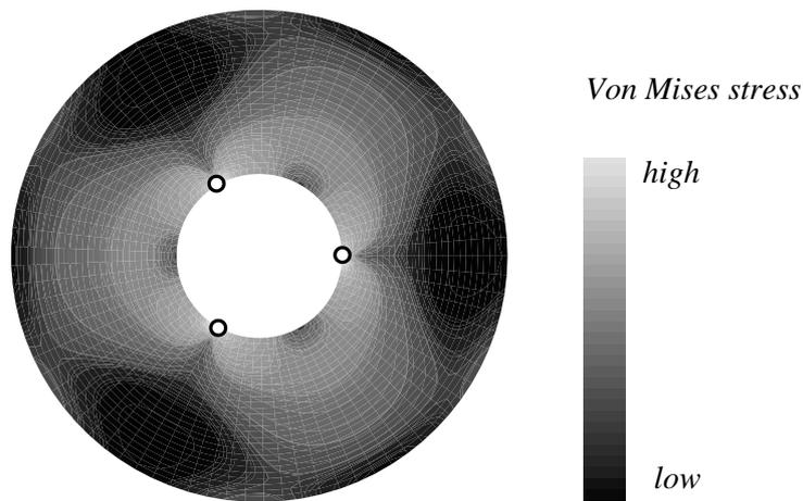
**Fig. 6.** Stress distribution in the initial disk.
