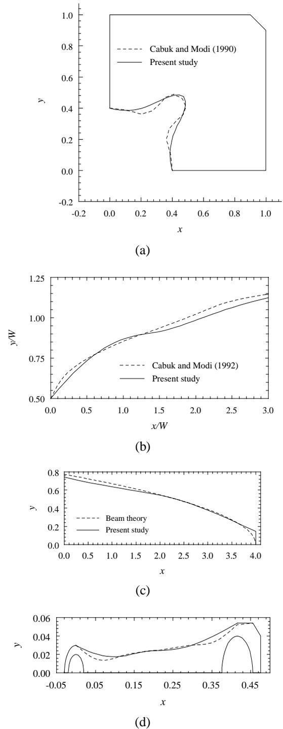
Figure 16. (a) Optimum 90-degree elbow compare to Cabuk and Modi (1990), (b) Optimum diffuser compare to Cabuk and Modi (1992), (c) Optimum cantilever beam compare to the result from beam theory (Eq. (10)), (d) Optimum torque arm compare to the result from Richards (1995) (dashed line).
