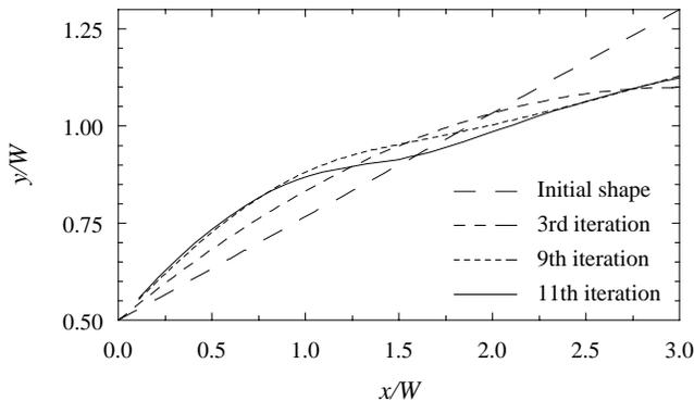
Figure 9. Evolution toward the optimum diffuser.
