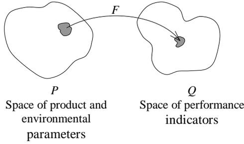
**Figure 1. A mapping for a mathematical abstraction of robustness in design.**
