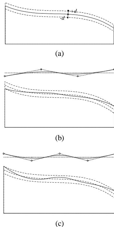
**Figure 5. (a) Designed shape and tolerance envelope, (b) 4-control point quadratic B-spline curve overlapping the designed shape, (c) 5-control point quadratic B-spline curve overlapping the designed shape.**
