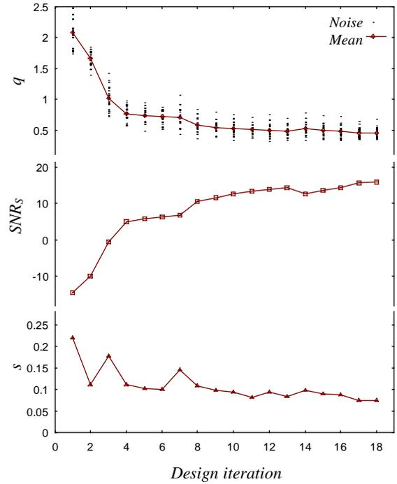
Figure 7. Variation of objective function mean along with the noise on  $q$ ,  $SNR_S$  and  $s$  with design iteration.
