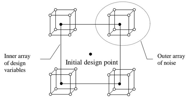
**Figure 3. Crossed arrays for robustization.**
