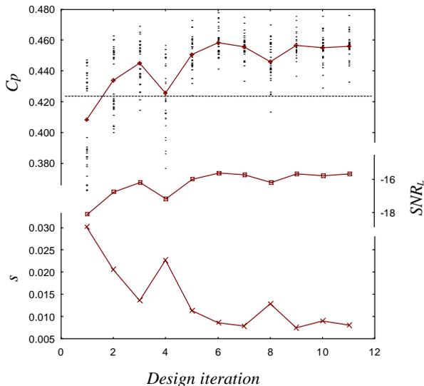
Figure 10. Variation of mean along with the noise on  $C_p$ ,  $SNR_L$  and  $s$  with design iteration.
