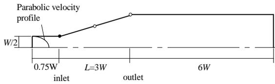
Figure 8. Plane symmetric diffuser.
