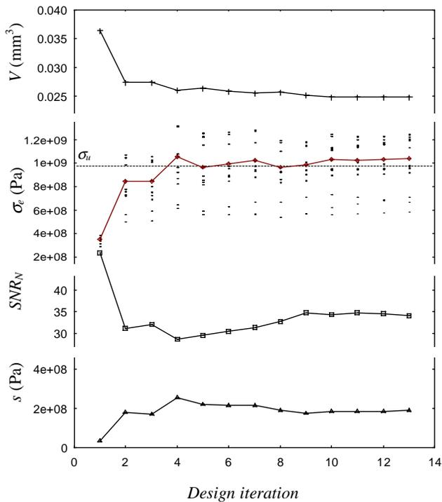
Figure 15.  $V$ , Variation of mean along with the noise on  $\sigma_e$ ,  $SNR_N$  and  $s$  with design iteration.
