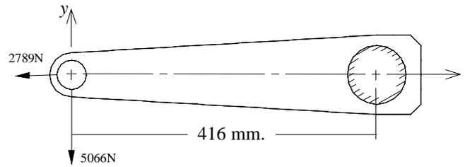
**Figure 13.** Torque arm.
