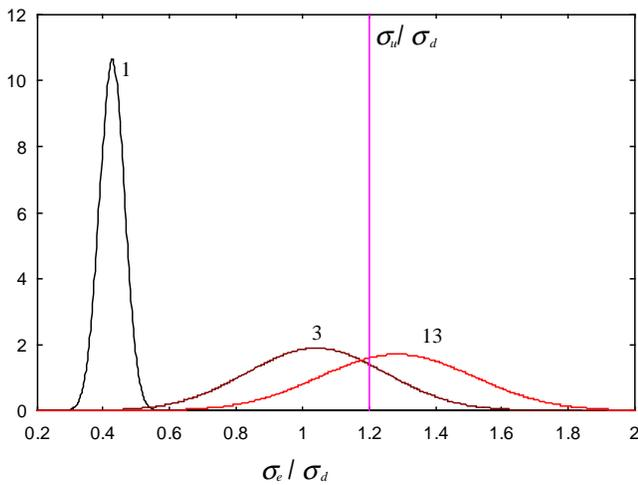
Figure 19. Normal distribution of stress of some torque arm designs
